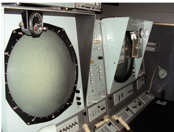
Konsole operatorskie radaru RSP-6/M2
